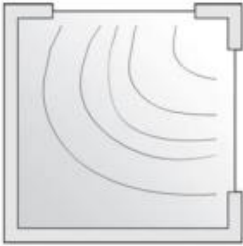
Figure 8: Balanced lighting Distribution by Two Adjacent Side Windows.
