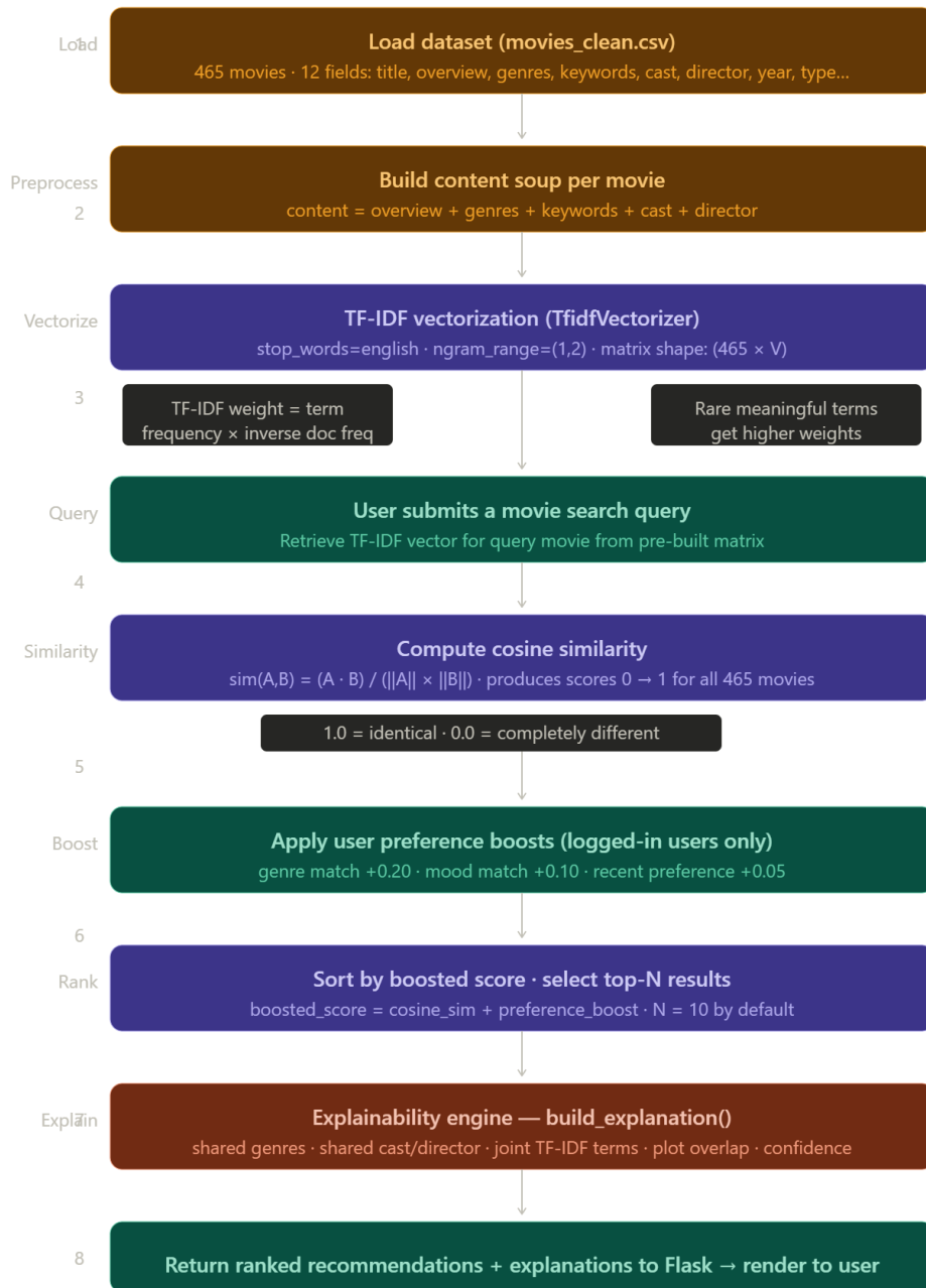
Figure 3.1 System algorithm diagram of the proposed system
