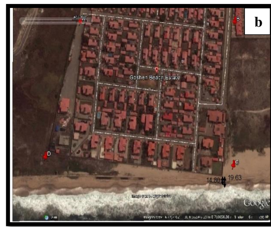
Plate 3.1a, b. Goshen Estate in 2012 and 2013 showing distances of the fence from the coastline. Note the beach configuration before the construction of groins; a. Goshen Estate in 2012 showing distance of fence from the coastline -19.63m & wet/dry line - 14.80m; b. in 2013 showing distance of fence from coastline – 16.05m & wet/dry line – 11.21m (after erosion/ocean surge of July 2012 (Imagery source: Google Earth, 2012 & 2013).
