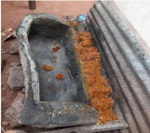
Ikwe Ekwu – Long wooden mortar for palm oil processing
