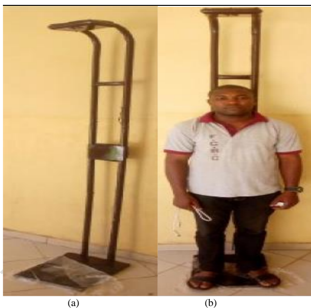
Fig. 12: The proposed automatic BMI machine: (a) shows the isometric view and (b) BMI measurement with the BMI machine.
