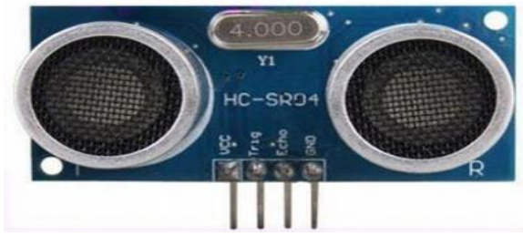
Figure 2. The HC-SR04 ultrasonic proximity sensor
