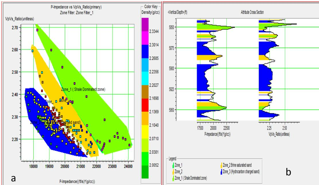
Fig.4. (a) Crossplot of velocity ratio and P-Impedance (b) Attribute Cross-Section showing hydrocarbon, Brine and Shale intervals
