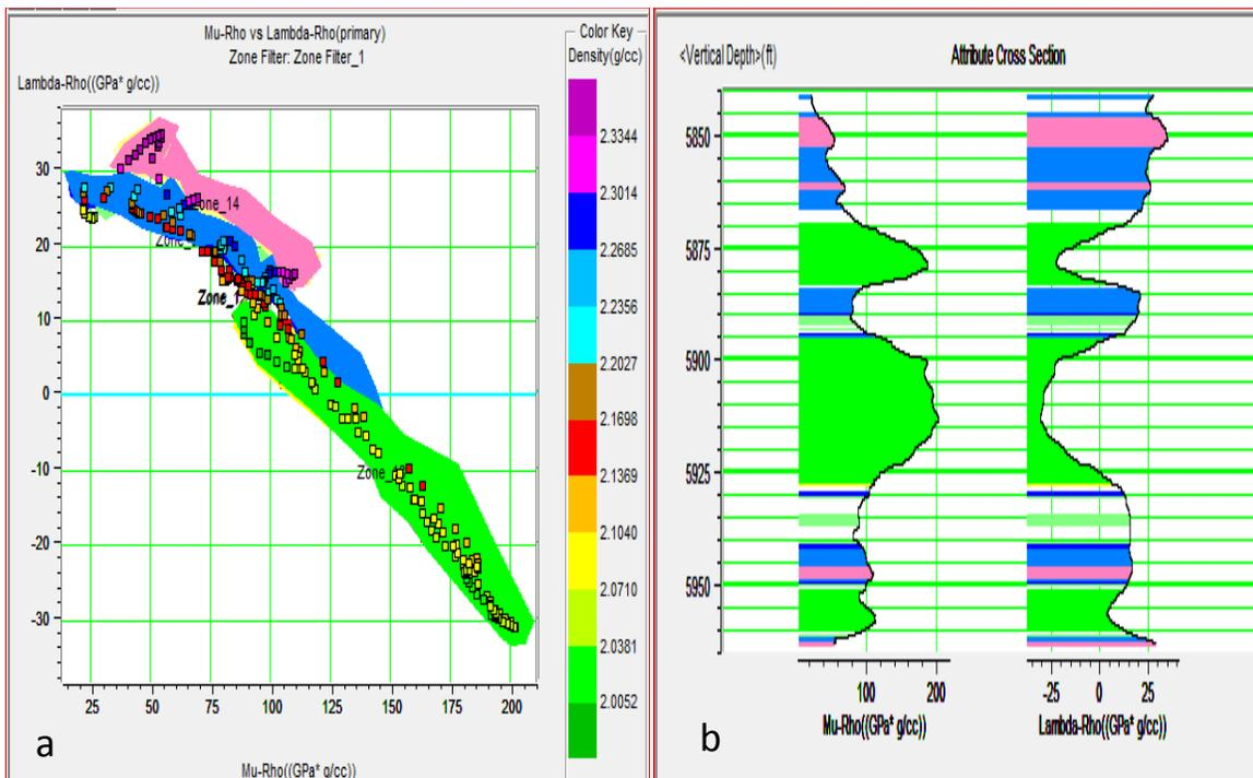
Fig.5. (a) Crossplot of LamdaRho ( $\lambda * \rho$ ) and Mu-Rho ( $\mu * \rho$ ) (b) Attribute Cross-Section MuRho ( $\mu * \rho$ ) and LamdaRho ( $\lambda * \rho$ ) showing Gas, Brine and Shale intervals
