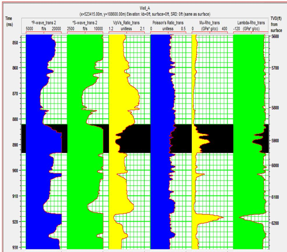
Fig.2. The generated well log attributes indicating HD2 reservoir
