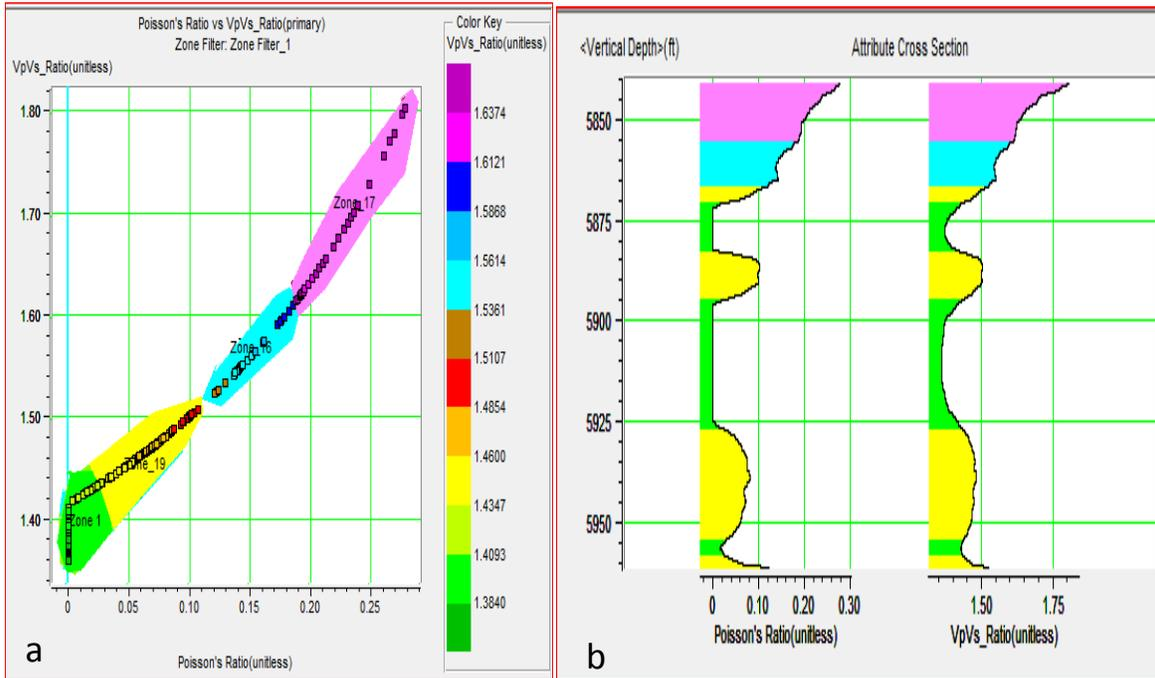
Fig.3. (a) Crossplot of velocity ratio and Poisson' ratio (b) Attribute Cross-Section showing hydrocarbon, Brine and Shale intervals
