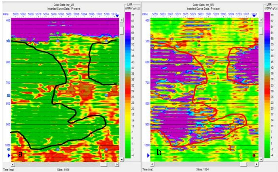
Fig.7. Lambda-Mu-Rho (LMR) inversion (a) Inverted LambdaRho volume (b) Inverted MuRho volume
