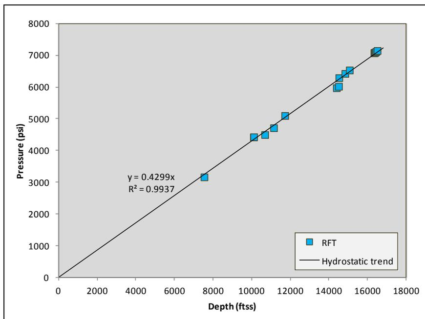
Figure 3 Plot of measured pore pressures in freely draining aquifers for the determination of suitable hydrostatic pressure baseline in the field. A gradient of 0.4299psi/ft ( $\approx 0.43$ psi/ft) was calculated for hydrostatic pressures and was used as the basis for quantifying excess pressures in the field.
